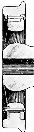
Figs. 5312-5213. Wheel for Engine-truck. Cast-iron Spoke-center. Tire secured by a Steel Retaining-ring. PAIGE CAR WHEEL COMPANY.
